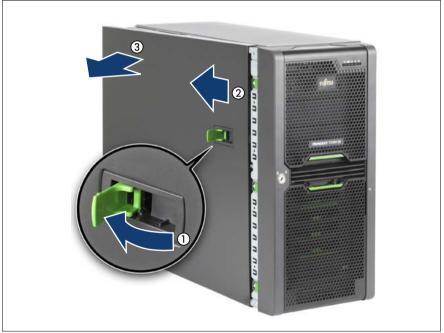
Figure 27: Opening the server (example: floorstand model)
